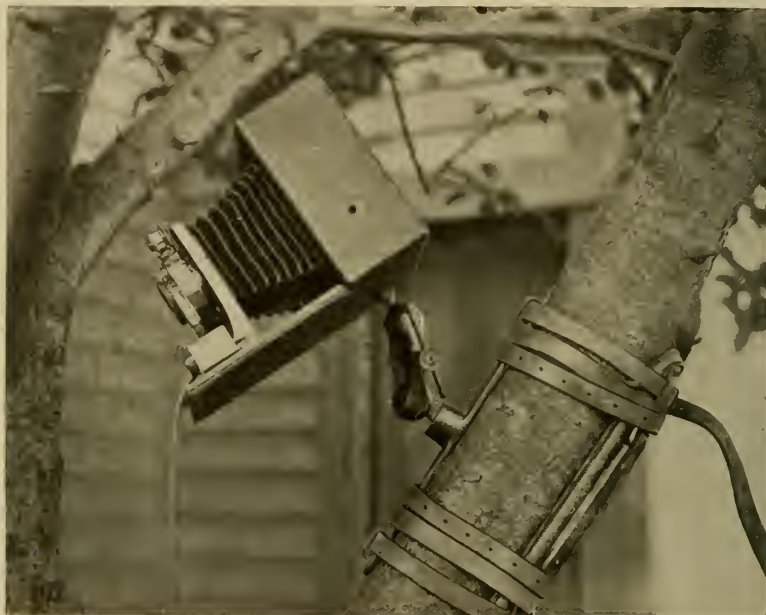
METHOD OF ATTACHING A SMALL CAMERA TO A LIMB
